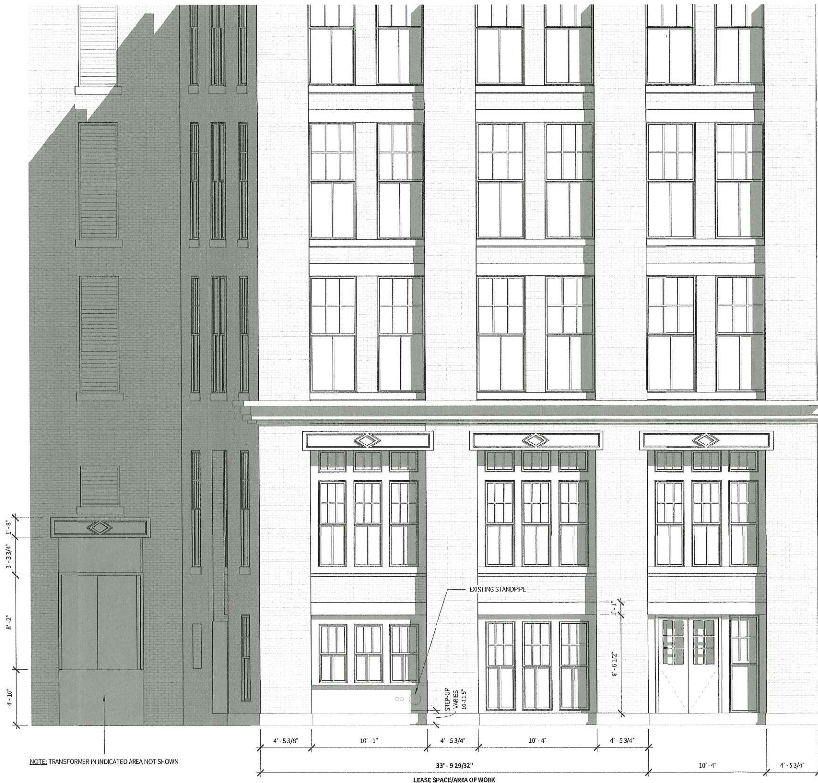
① EXISTING EXTERIOR NORTH ELEVATION 1/4" = 1'-0"
