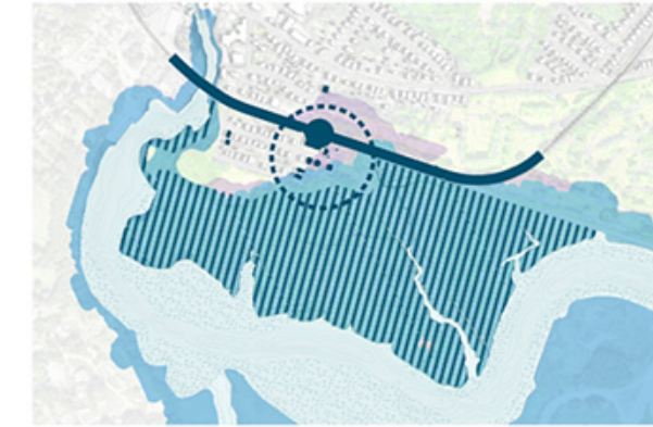
1% Annual Chance Flood with 40 in of SLR (2070s) with near-term and long-term coastal resilience solutions in place
