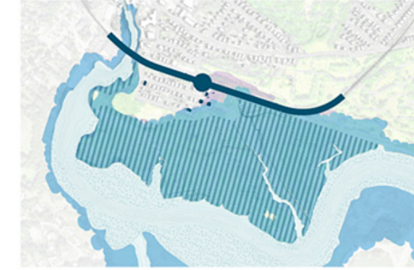
1% Annual Chance Flood with 9 in of SLR (2030s) with near-term coastal resilience solutions in place
