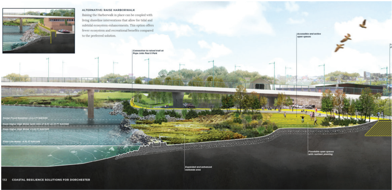
Figure 4-7. Section of Dorchester Illustrating Coastal Flood Protection, Climate Ready Boston (City of Boston, 2020)
