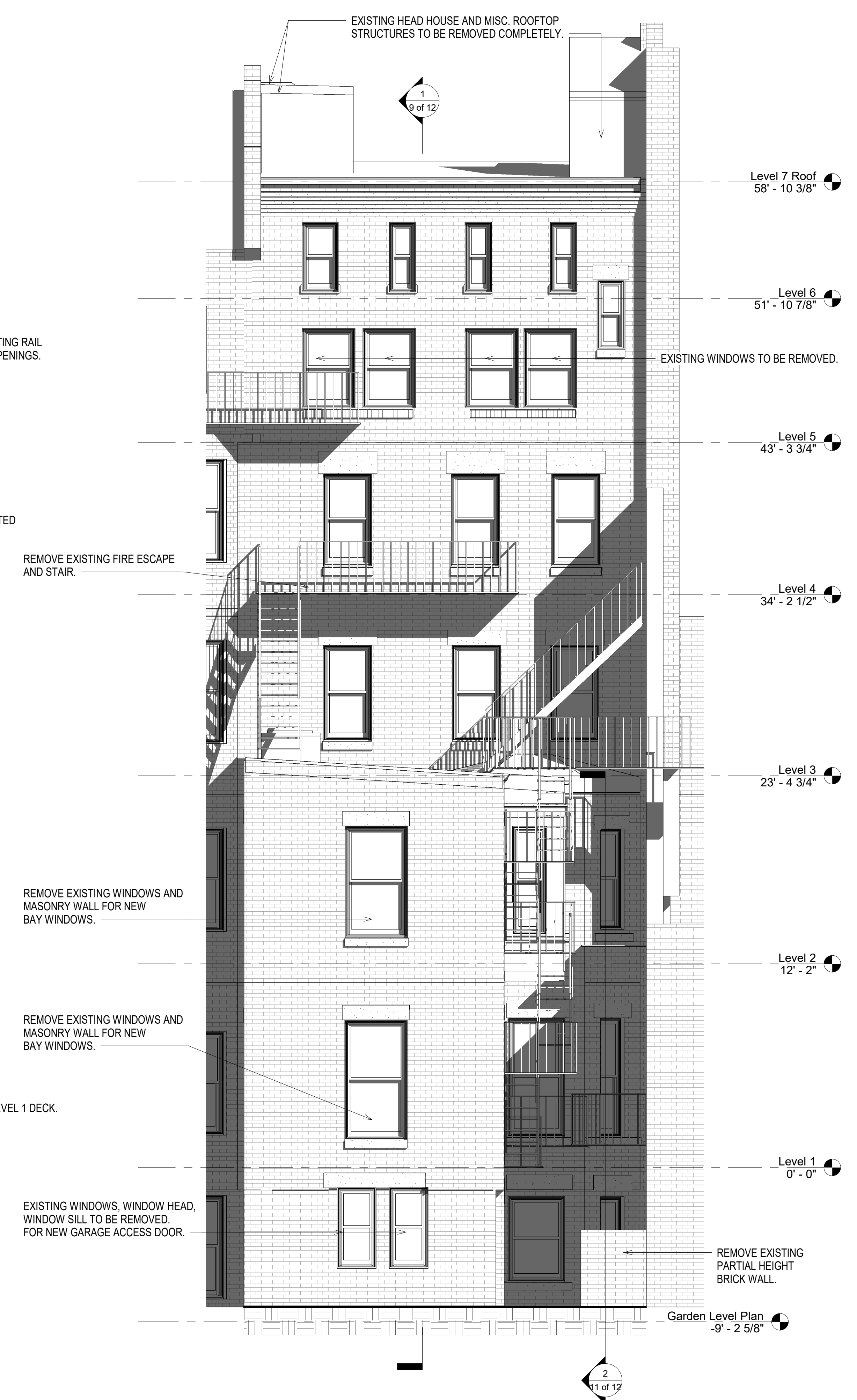
② Existing West Elevation 1/4" = 1'-0"
